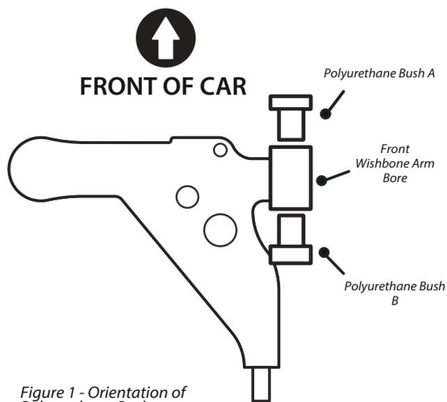
Figure 1 - Orientation of Polyurethane Bushes
